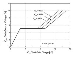
Figure 6. Gate Charge Characteristics
