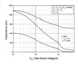
Figure 5. Capacitance Characteristics
