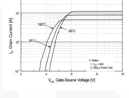
Figure 2. Transfer Characteristics
