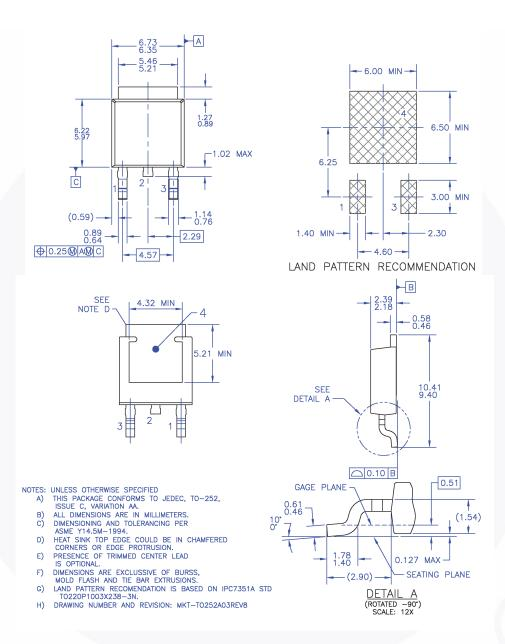
Figure 16. TO252 (D-PAK), Molded, 3 Lead, Option AA&AB
