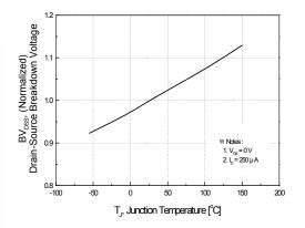
Figure 7. Breakdown Voltage Variation vs Temperature
