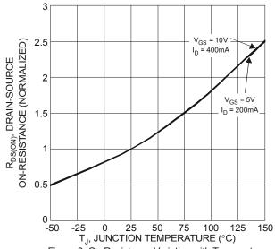
Figure 6 On-Resistance Variation with Temperature
