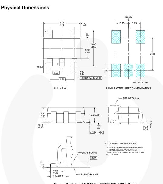
Figure 7. 5-Lead SOT23, JEDEC MO-178 1.6mm
